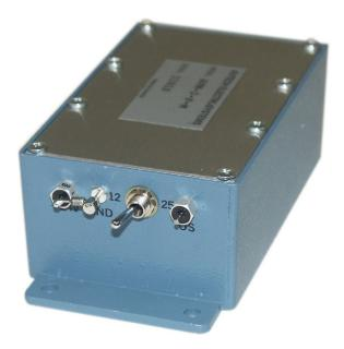
The "12/25" switch should be set in the "12" position if the PRF is less than 12 MHz. For higher PRF the switch should normally be in the "25" position for optimal rise times and pulse widths.
